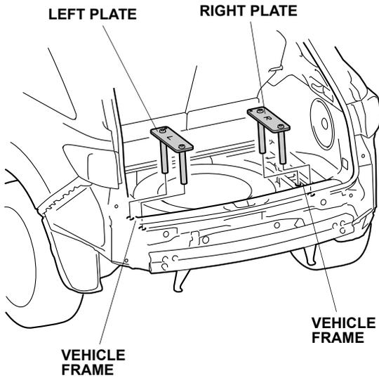
13. With the help of an assistant, insert two spacers between the trailer hitch and the vehicle frame. Mount the trailer hitch using two loosely-installed 12 x 40 mm bolts with spring washers and plain washers. Be careful that the spacers do not fall out during installation.
