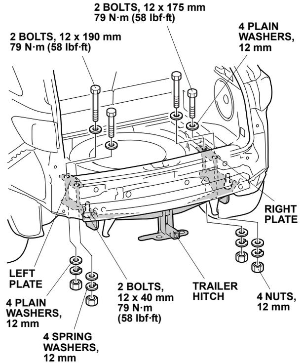
15. Tighten the 12 x 40 mm bolts installed in step 13. Then tighten the 12 x 190 mm bolts and the 12 x 175 mm bolts. Torque all of the 12 mm nuts and bolts to 79 N·m (58 lbf·ft).
